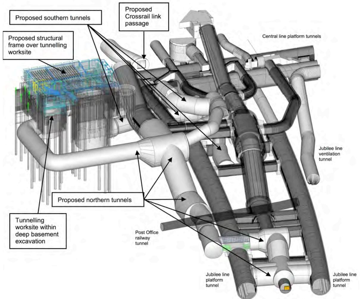
Figure 2 Overview of existing and new (light colour) underground structures
